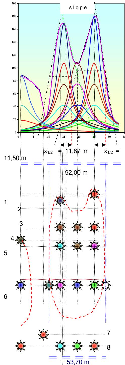
Figure 13. Profile verification of field data with modeling to reconstruct of target (I - J slice)
