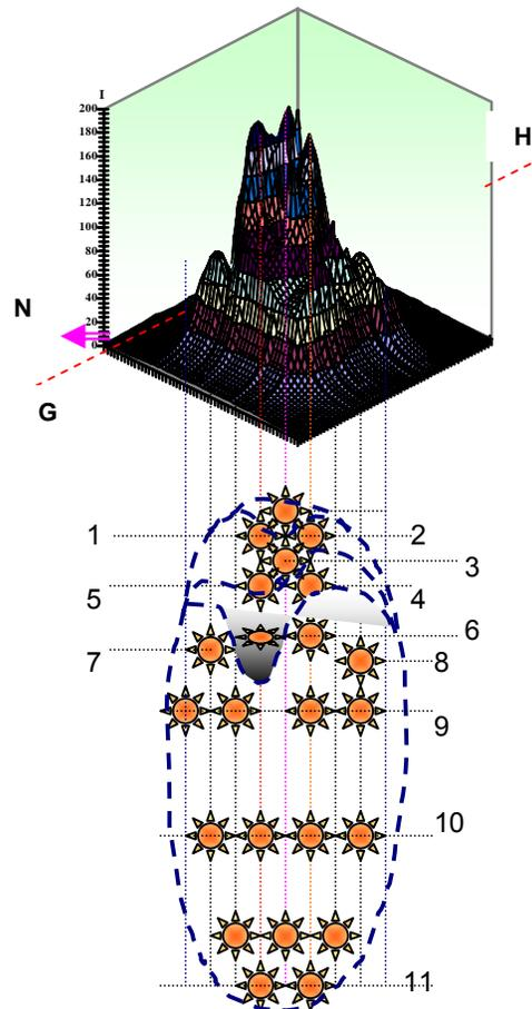
Figure 17. Curve of radiation intensity in three dimensions to reconstruct of target that is adjusted with two dimensions curve on contour G – H slice
