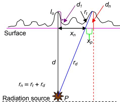
Figure 2. The shape of modeling geometry to calculate radiation intensity that it's profile may be in mutual accord with profile of field data on topography correction
