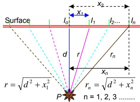
Figure 1. The shape of modeling geometry to calculate radiation intensity that it's profile may be in mutual accord with profile of field data on elevated or altitude correction
