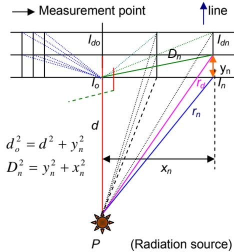
Figure 3. The shape of modeling geometry in three dimensions to calculate radiation intensity that its profile may be in mutual accord with profile of field data on elevated correction
